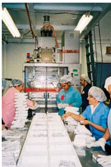
Operators hand-pick filled stick-packs of granular product as they exit the vf/f/s machine in groups of six.
